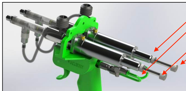
Pict. 5.3: Adjusting the quantity of drug to be injected
